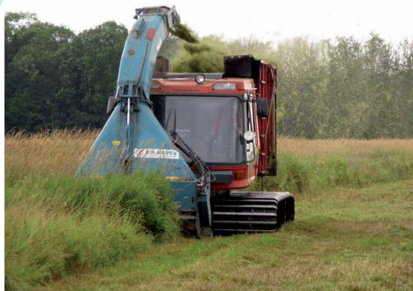
Fig. 1: Harvest of gramineous biomass on a rewetted peatland with a tracked vehicle.
