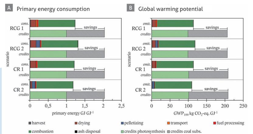
Fig. 3: Primary energy consumption (A) and global warming potential (B) differentiated by scenarios and life cycle stages. Expenses (upper bar) and credits (lower bar) referring to environmental burden or relief. The difference between total expenses (consumption/emissions) and credits indicates the savings compared to hard coal firing. RCG - Reed Canary Grass, CR - Common Reed, cons. - consumption, emit. - emissions.
